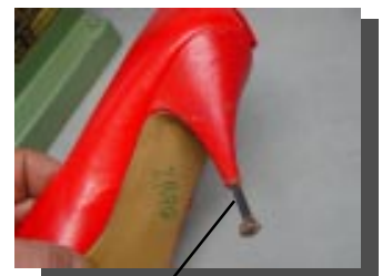
Top Lift Pin Removed from Heel Base
