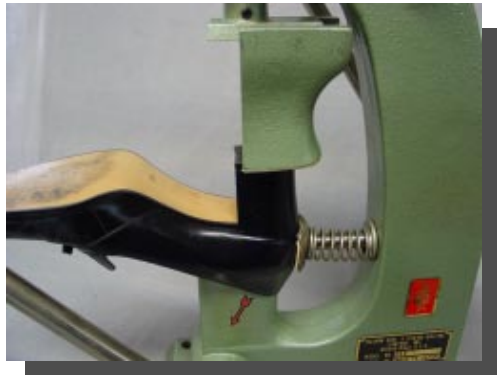
Spring Loaded Plate Holds Shoe in Place
