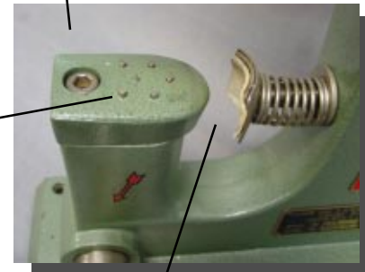
Spring Loaded Plate Holds Shoe in Place
