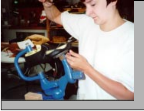
Hand Sewn Moc Toe, a student stitching directly on the shoe last.
