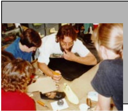
Pattern Design Directly on the Shoe Last.
